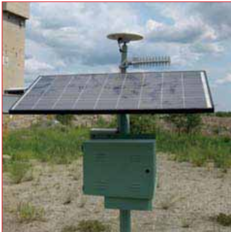
Figs. 7 and 8: The GPS receivers and wireless access points are powered by solar power.
