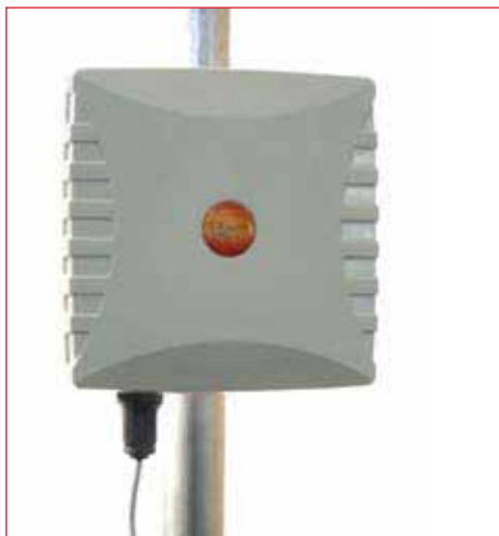
Fig. 5 and 6: Directional antenna at TIM installation 2,4 GHz, 15 DBi gain antenna 30° x 30° beamwidth.
