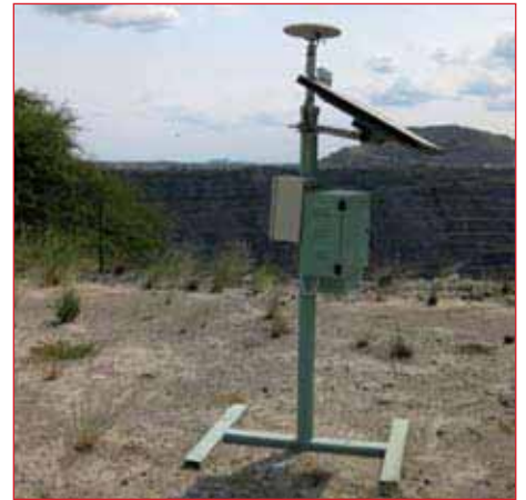
Fig. 9: If the objective is to detect millimetre movement or trends, this becomes virtually impossible when utilising a mobile installation.
