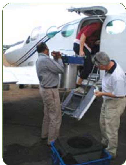
Fig. 7: A modern digital mapping camera being installed in Cessna Golden Eagle CIII in 2008. (Image courtesy of Geospace International – Bernhard Jacobs).
