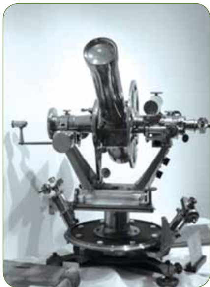
Fig. 2: Repsold theodolite 254 mm (10 inch) used by Sir David Gill circa 1890 on display in the CD:NGI Museum.
