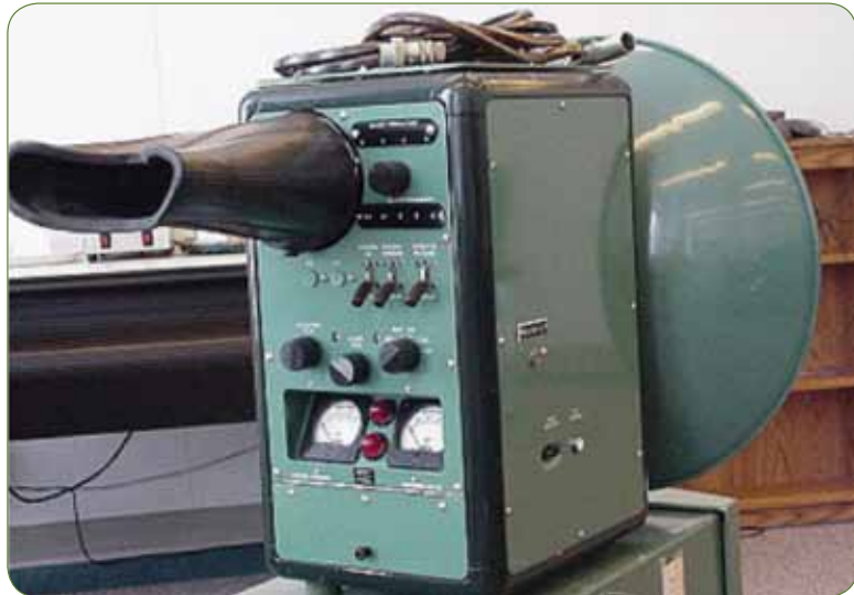
Fig. 4: Early Tellurometer MRA 1.
