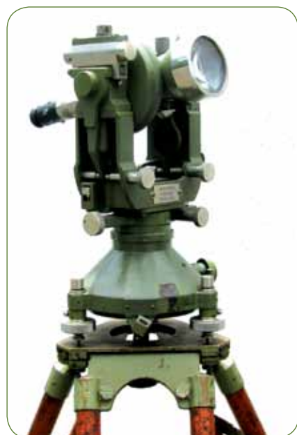
Fig. 3: "Wild T3 104 mm (5 1/2 inch) geodetic theodolite on display in the NGI museum. The maker's plate reads "Heinrich Wild, Heerbrugg, Schweiz, No 1."
