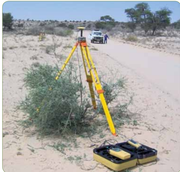
Fig. 5: GPS receiver being used for the survey of photo control in the Kgalagadi 2009 (Image courtesy of Gerhard Visser).
