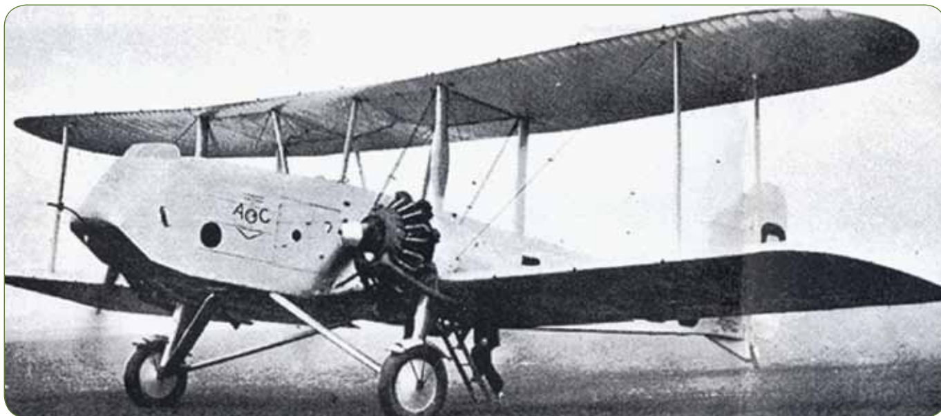
Fig. 6: Gloster A.R 24 Survey aircraft used for aerial photography by the Aircraft Operating Company circa 1931. Note camera operators open cockpit at front of aircraft. Only two such aircraft were built. (Image courtesy of AOC Geomatics – Chris Tanner).
