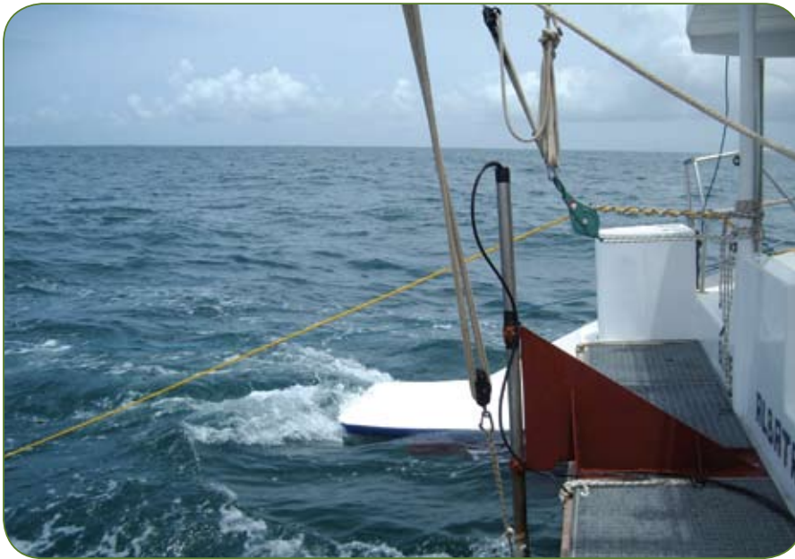
Fig. 3: Echosounder pole and SSS tow cable.
