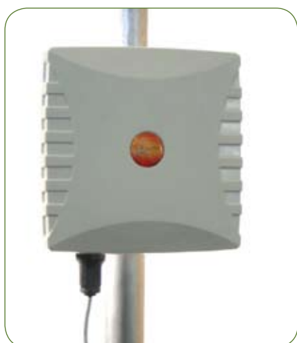
Fig. 5 and 6: Directional antenna at TIM installation 2,4 GHz, 15 DBi gain antenna 30° x 30° beamwidth.
