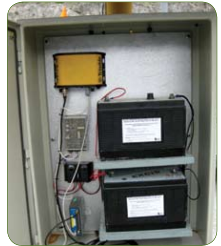
Figs. 7 and 8: The GPS receivers and wireless access points are powered by solar power.
