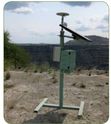
Fig. 9: If the objective is to detect millimetre movement or trends, this becomes virtually impossible when utilising a mobile installation.
